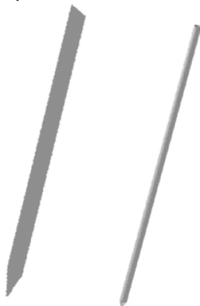
Fig. (2). Blade electrode with 5 \times 0.1 mm cross section (left), and needle electrode with 1.2 mm (18 gauge) diameter (right), both 50 mm long.
